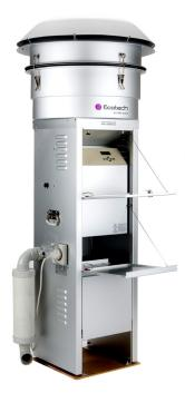
The HiVol 3000 particulate sampler performs remote unattended sampling of  $PM_{2.5}$ ,  $PM_{10}$  or TSP along with basic meteorological parameters.
