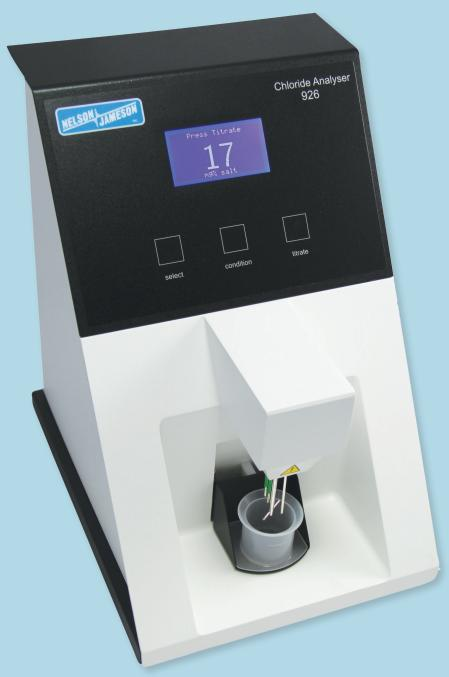
The Nelson-Jameson 926 Chloride Analyzer is a reliable, accurate, and exceptionally easy to use instrument dedicated to the measurement of total chloride with a feature to determine percent salt. This includes a broad spectrum of food products, raw materials, and industrial applications. At the touch of a button, you can have results displayed directly as mg/1 (ppm) or mg % salt.
